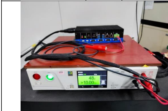
Insulation resistance test after Damp Heat Test (DC terminal to metal enclosure )
