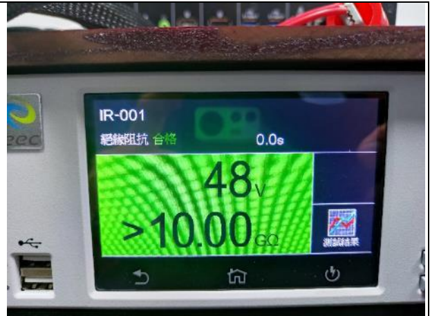
Insulation resistance (DC terminals to metal enclosure)
