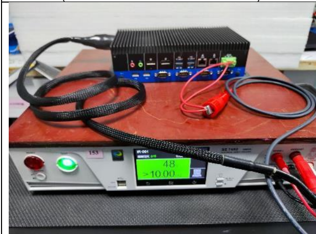
Insulation resistance test after High Voltage Test (DC terminal to metal enclosure)
