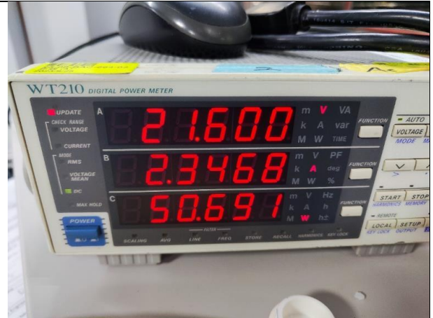
During the 2 hours Performance check with Extreme power supply -10%
