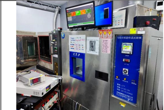
During the last 2 hour doing performance test (21.6Vdc)
