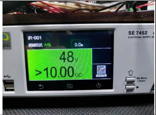
Insulation resistance (DC terminals to output connectors)
