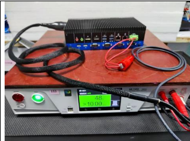
Insulation resistance (DC terminals to metal enclosure)
