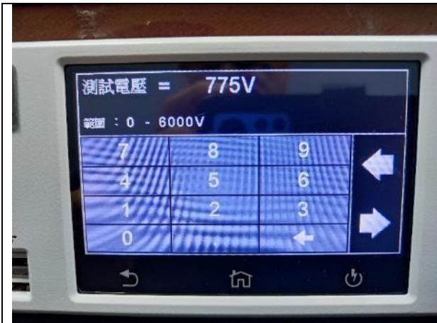
Setup test voltage 775Vdc
