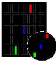
Cluster pixel defect type 3a Sub-pixels/dots in a cluster area constantly lit
